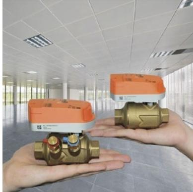
The new PIQCV (Pressure Independent Quick Compact Valve) from the Belimo ZoneTight™ product range uses automatic and permanent hydraulic balancing to supply the precise amount of water required at all times to all of the heating and cooling elements, providing ideal room comfort. These valves are compact, flexible and efficient.
