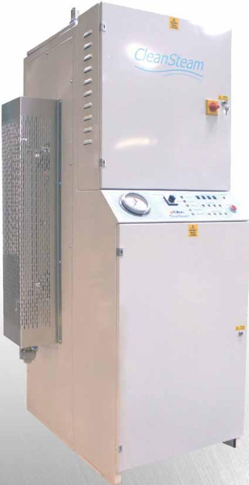
The CleanSteam combined steam boiler, has a large thermal mass providing flash steam reserve. This enables the boiler to meet fluctuation in steam loads and to meet the short-term peak flow rates of a typical sterilizer cycle. The boiler is designed to reduce entrainment of water droplets to a minimum and, as a result, produce high quality, contaminant-free steam.
