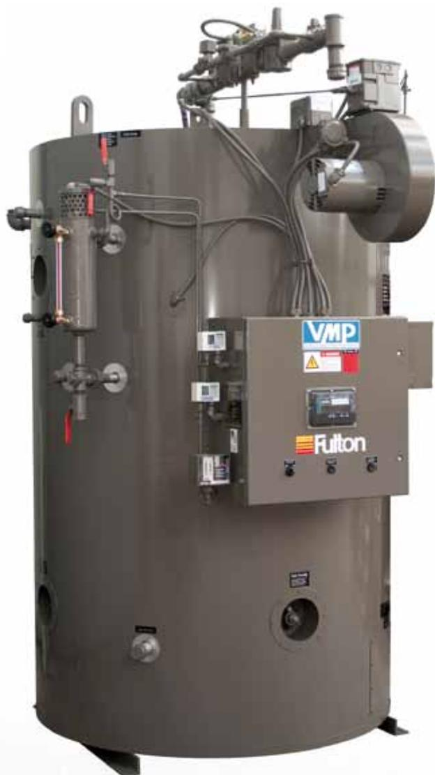
Within the Fulton VMP, a series of heavy walled large diameter schedule 80 flue pipes are welded to the top and bottom heads in the pressure vessel and these pipes are surrounded by water. The water-backed design speeds up boiler start up time and creates overall even heating throughout. This, along with many other design features of the VMP, result in fuel to steam efficiencies of up to 84%.
